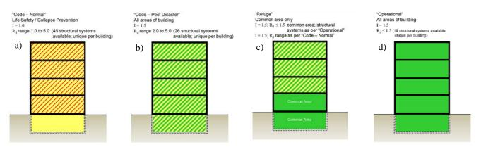
Figure 1. Performance levels: a) Code-Normal, b) Code-Post Disaster, c) Refuge, d) Operational.
