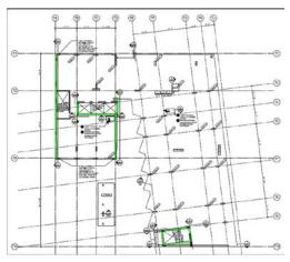
Figure 5. Typical floor plan of the building highlighting (in green) concrete shearwalls as SFRS.
