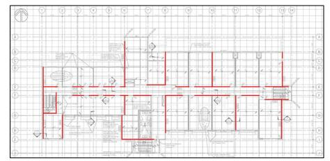
Figure 3. Typical upper floor plan of the building highlighting (in red) nailed plywood shearwalls as SFRS.
